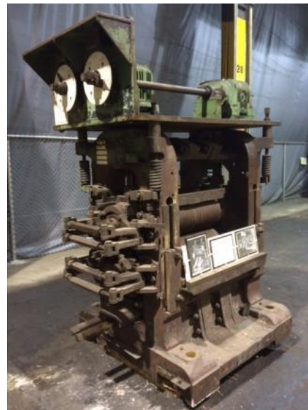
Continuous 12" Mill, installed 1943, Stand 14 on display in Bldg. 140. Approx. 4'x4'x8' 14,000 lbs.
