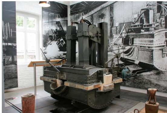
1905 – Héroult electric-arc furnace [4]
